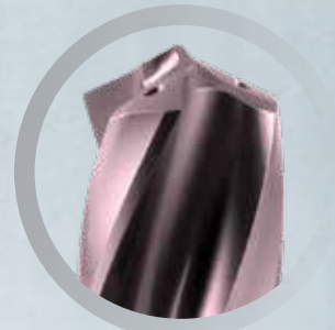
pyramid-shaped tip prevents radial deflection while entering the workpiece
